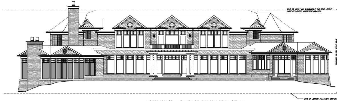
2 MAIN HOUSE - SOUTH EXTERIOR ELEVATION 1/8" = 1' - 0"
