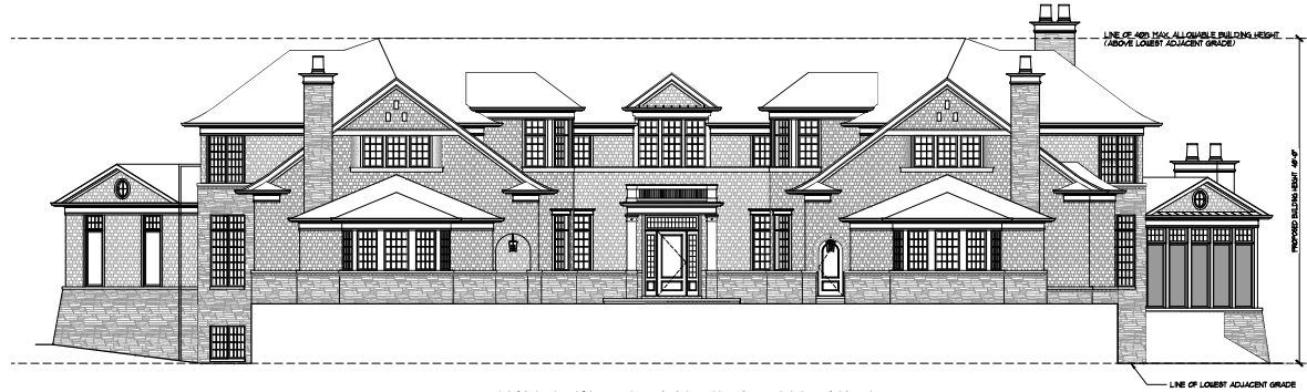
1 MAIN HOUSE - NORTH EXTERIOR ELEVATION 1/8" = 1' - 0"
