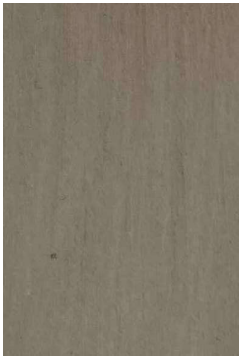
CEDAR WALL SHINGLES NO.1 CLEAR R&R WESTERN RED CEDAR W/ 5" EXPOSURE FOR STAIN; SEMI-TRANSPARENT GRAY
