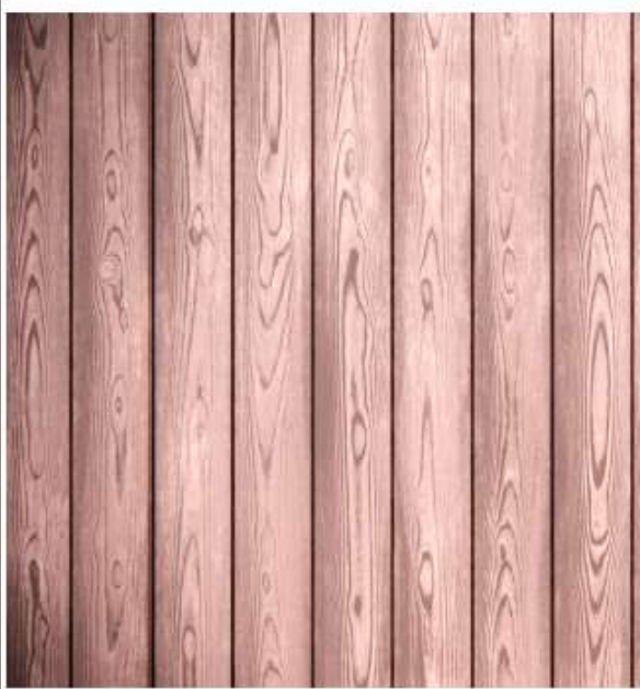
BARNWOOD, WEATHER AGED ROUGH SAWN VERTICAL SIDING - 3" BOARDS WEATHERPROOF RED STAIN MILLED BUTT JOINTS WITH 1/4" DARK STAINED REVEAL REFERENCE RENDERINGS FOR COLOR LOCATION
