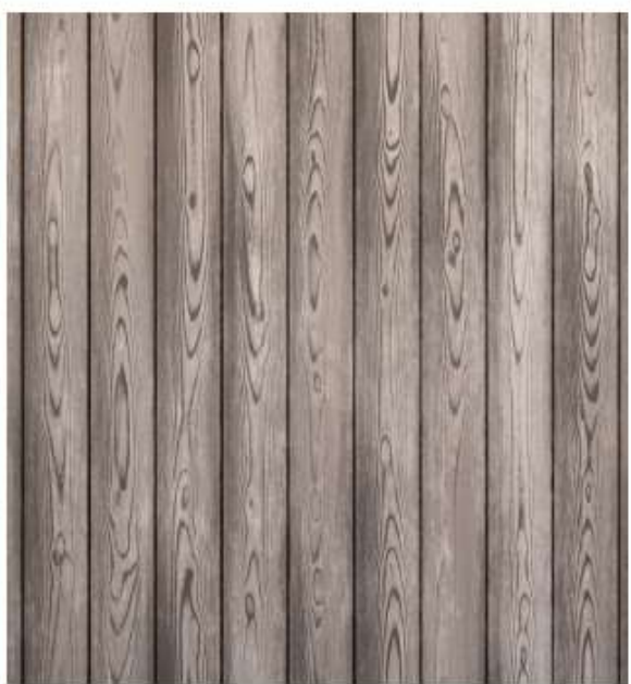
BARNWOOD, WEATHER AGED ROUGH SAWN VERTICAL SIDING - 3" BOARDS WEATHERPROOF GRAY STAIN MILLED BUTT JOINTS WITH 1/4" DARK STAINED REVEAL REFERENCE RENDERINGS FOR COLOR LOCATION
